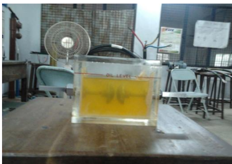
Fig 2: Semiconductive Nanofluid sample used for AC breakdown test
