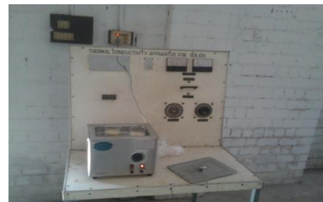
Fig 1: Ultrasonic Agitator used for Preparing Nanofluids
