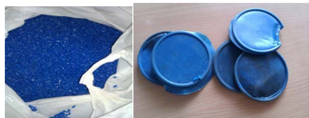
Fig. 2: PVC granules and PVC and Fly-Ash Composite Billets
