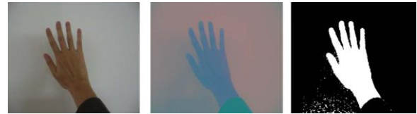
Figure 5: Example Showing Conversion from Original Image to Binary Image. We can Convert RGB to YCrCb Color Space and Segment Hand Region from Original Input Image. (a) RGB Image. (b) YCbCr Image. (c) Binary Image
