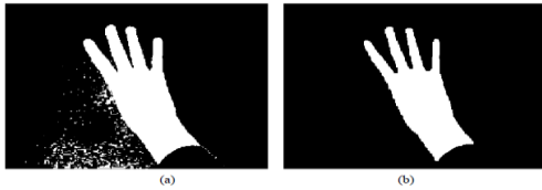
Figure 8: Example Showing the Result of Image Morphology. Perform Erosion and Dilation on Binary Image. (a) Original Image. (b) The Result of Image Morphology
